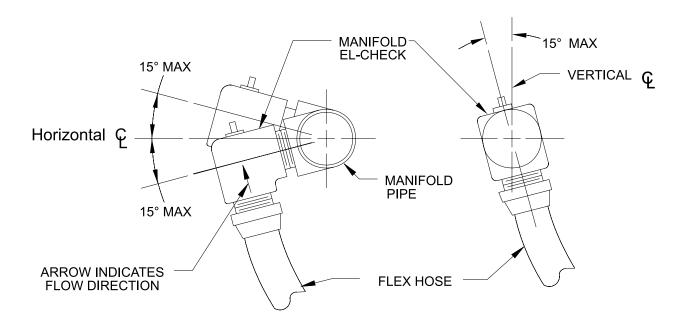
EL-CHECK MAY BE ADJUSTED AS SHOWN TO OBTAIN A SMOOTH RADIUS IN FLEXIBLE DISCHARGE HOSE.
