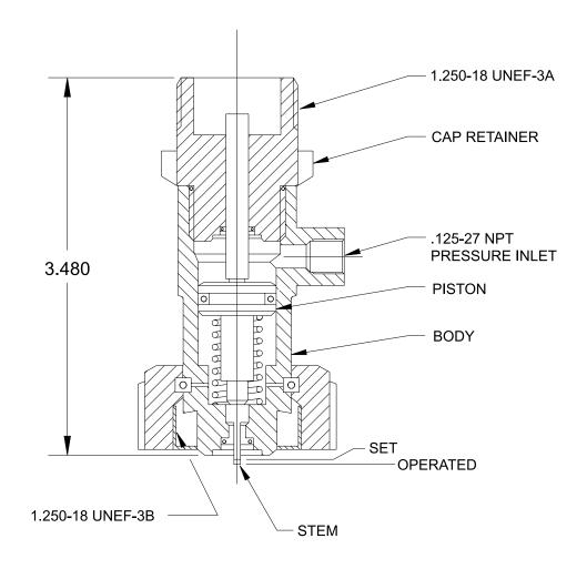
**MATERIAL** BODY, RETAINER CAP, PISTON & MTG. NUT: BRASS
