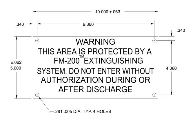
MATERIAL: ALUMINUM TYPE 1100-H14 OR 3003-H14, .032 ± .003 THICK. ALL LETTERS TO BE 48 PT. ALTERNATE GOTHIC#2. ETCHED .003 - .005 & FILLED IN WITH RED CHIP PROOF ENAMEL COLOR NO. 21105 PER FED. STC. 595 FINISH: ONE COAT CLEAR LACQUER BOTH SIDES
