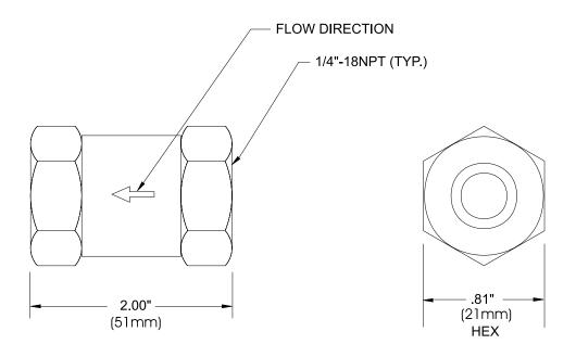
NOTE: INSTALL VALVE WITH ARROW POINTING IN DIRECTION OF FLOW.
