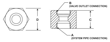
Note: For direct connection of cylinder valve to distribution piping.
